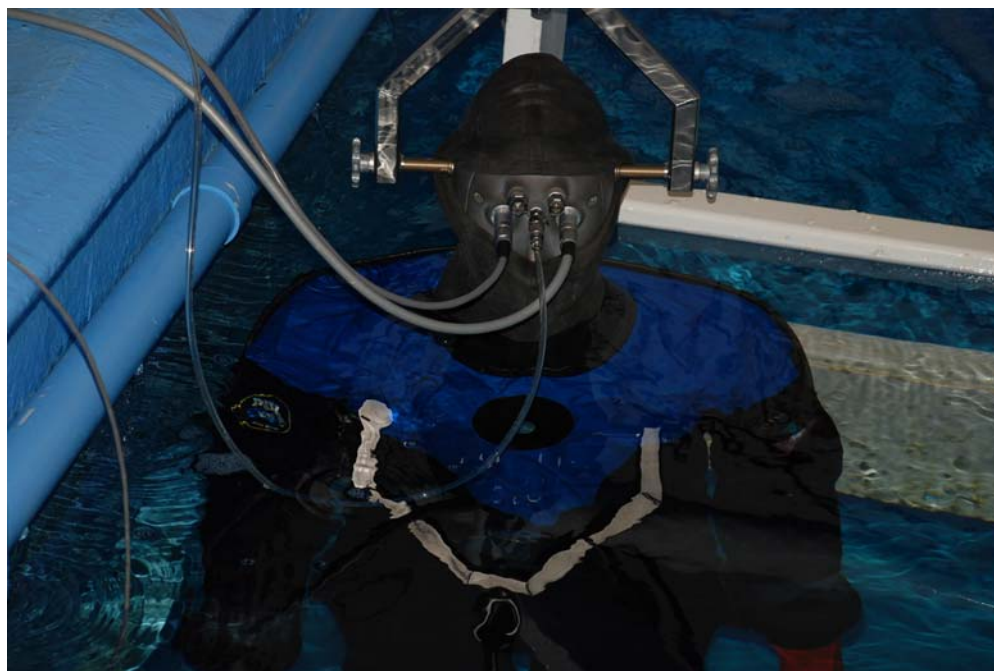
Fig. 5 Manikin submerged in a constant temperature test pool to neck level.
