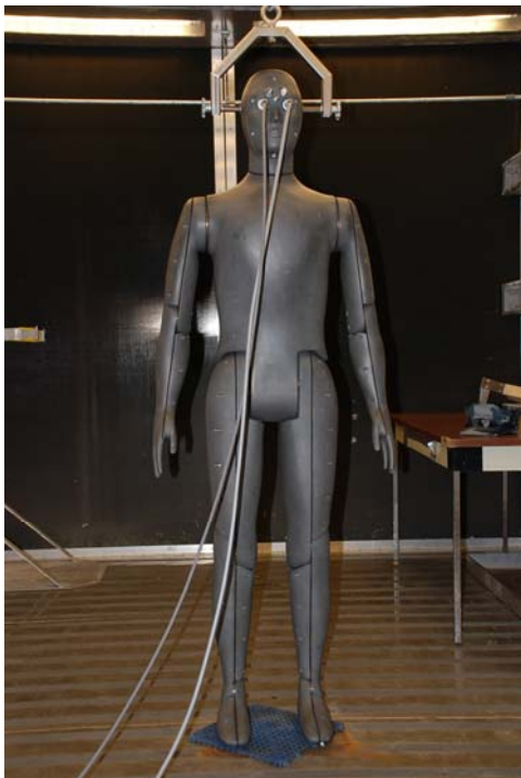
Fig. 2 21-zone thermal manikin used in testing at the Navy Clothing and Textile Research Facility in Natick, MA.
