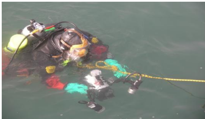
Figure 12. An EPA diver conducts a video transect on a bottom dumping site. Both surface and diver observations are recorded during the survey.
