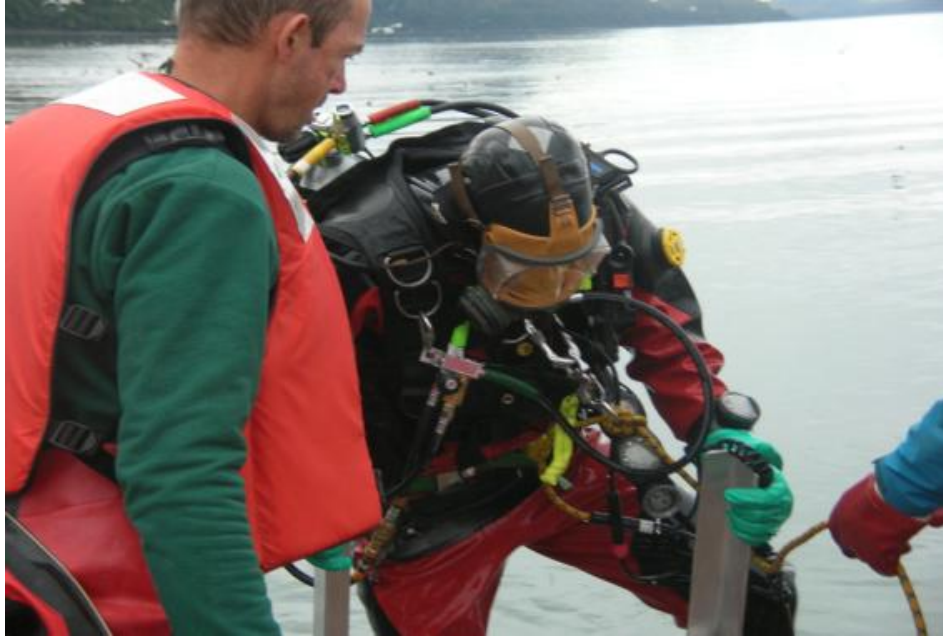
Figure 9. An EPA diver exits the water. Note the manifold block at picture center allowing the full face mask to be fed air from the primary or EGS tanks as needed.
