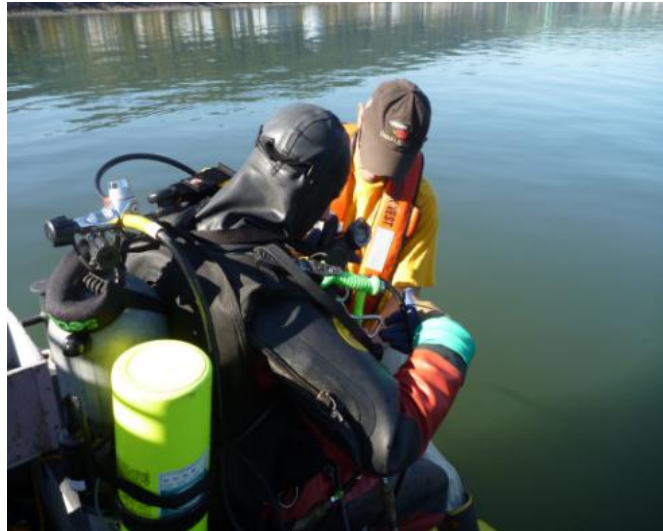
Figure 4. A yellow 30 ft 3 (cf) EGS bottle pictured on an EPA Superfund Site sampling project on the Willamette River, Oregon.
