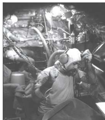
Fig. 4. Two diver-subjects after rapid compression to 800 fsw equivalent. Subject in foreground is having evaluation of bone conduction auditory thresholds. Subject in background is preparing to exercise on bicycle ergometer to measure ventilation and gas exchange (32).
