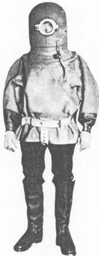
Figure 1. The Hall-Rees submarine escape breathing apparatus with built-in sodium peroxide oxygen generation [Fig 507 from Ref 4].
