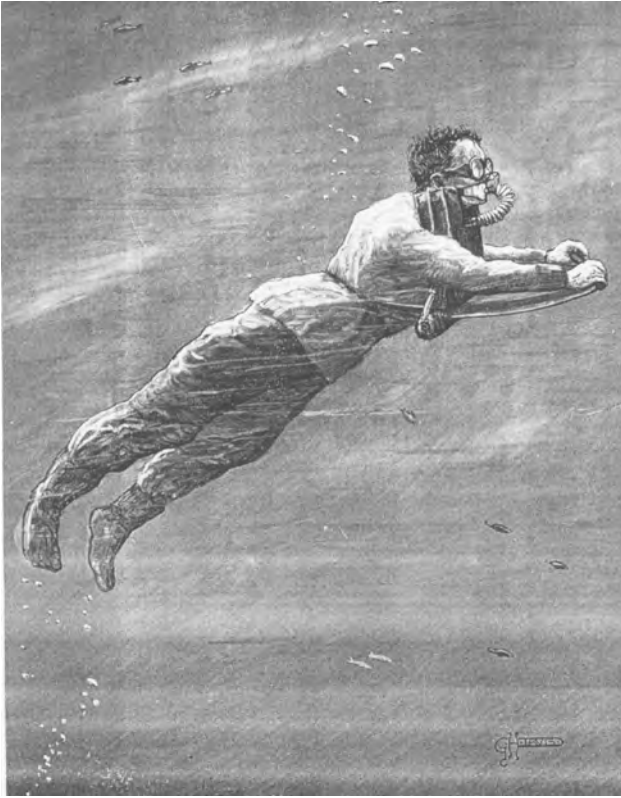
Figure 2. Davis submarine escape apparatus (DSEA) with vane extended to slow the rate of ascent. [Fig 252 from Ref4].
