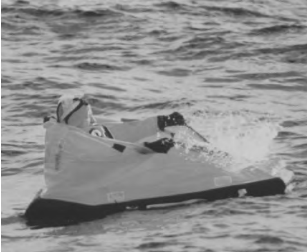
Figure 1. A “survivor” on the surface on the surface in the Mk 10 escape suit with the life raft inflated.
