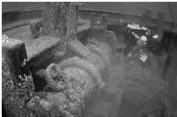
Figure 4. The windlass showing the Norman Pin (inverted u-shaped metal in lower left). (photo by T. Thomsen)
